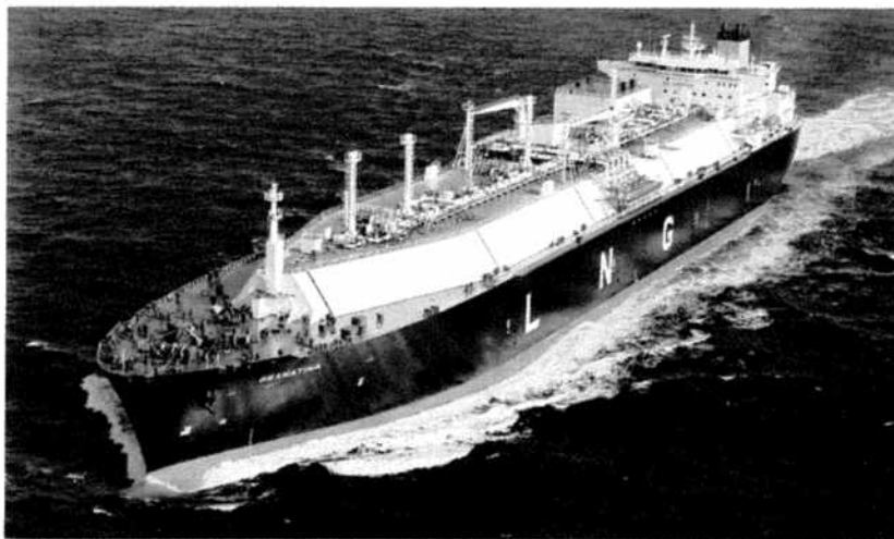
The three-year-old Granatina, sailing for Shell Gas & Power, is typical of the new generation of LNG carriers. Her 114,000-ton displacement supports more than 140,000 cubic meters of cargo.
